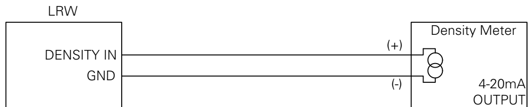
FIG. 3-19 DENSITY METER PROVIDES POWER FOR 4-20 mA DENSITY LOOP
